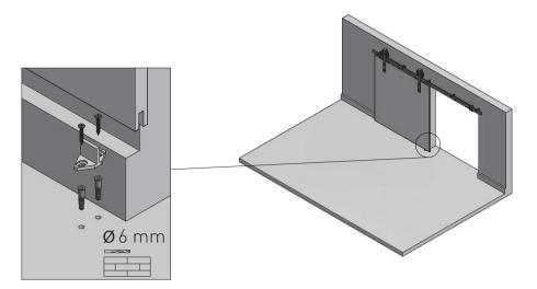
Stopper preventing door from falling out mounting
